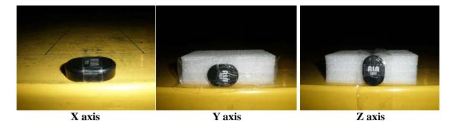
After verifying three axes, we found the maximum electromagnetic field was occurred at Y axis. The final test data was executed under this configuration.
