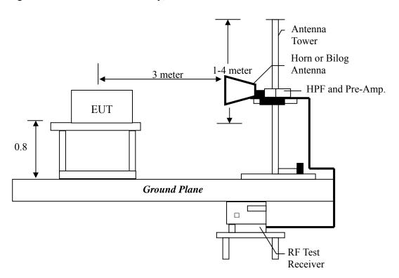
The signal is maximized through rotation and placement in the three orthogonal axes.
