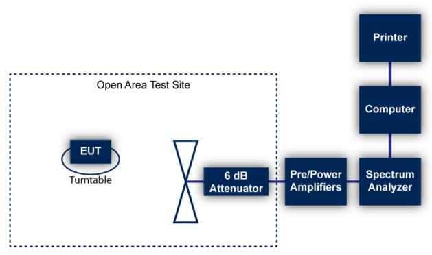
Figure 2: Radiated Emissions Test
