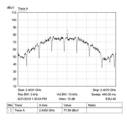
Graph 9: Lowest Channel 3 kHz PSD Plot
