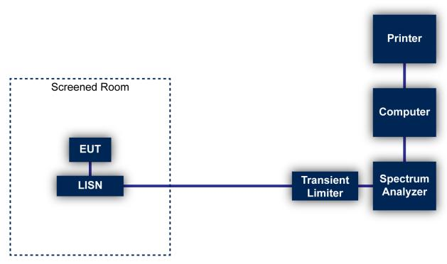
**Figure 1: Conducted Emissions Test**
