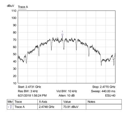
Graph 11: Highest Channel Output 3 kHz PSD Plot
