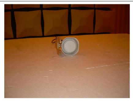
Photograph 3 – View Conducted Emissions On Edge Placement
