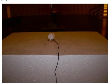
Photograph 2: Back View Radiated Emissions 30 MHz to 1000 MHz - Pointed Forward
