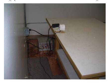
**Photograph 8 - Back View Conducted Emissions Worst Case Configuration**
