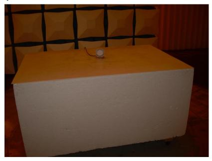
Photograph 1: Front View Radiated Emissions – Below 1000 MHz – Forward Pointed
