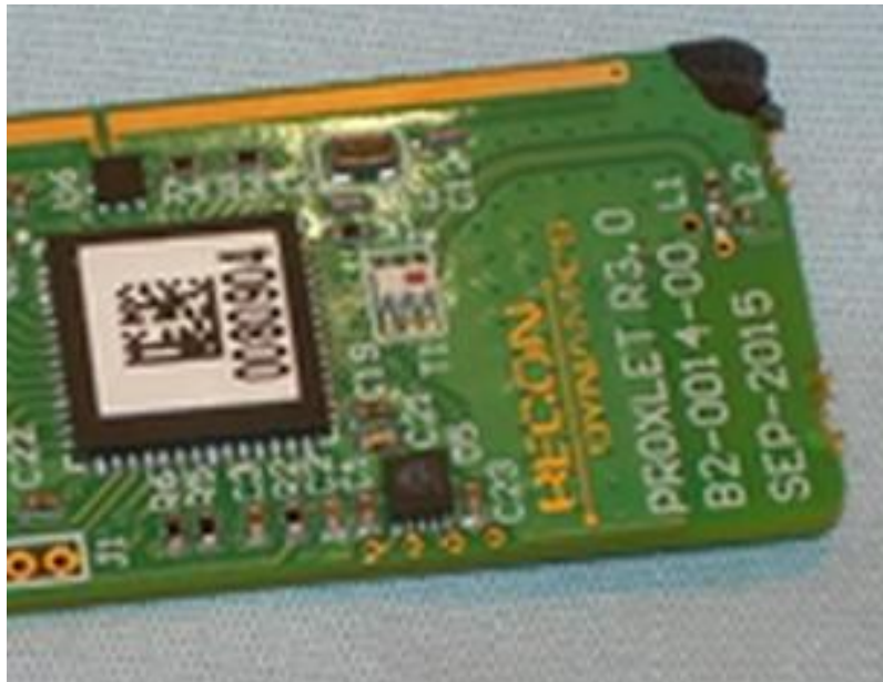
Photograph 9: RF Section of the Module with the Battery Removed
