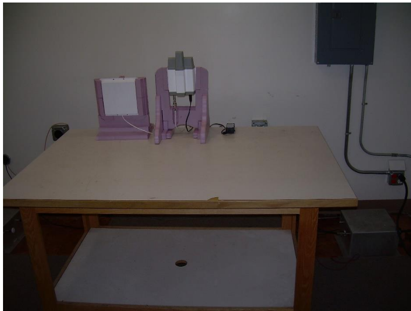
Photograph 8 – Front View Conducted Emissions Worst-Case Configuration
