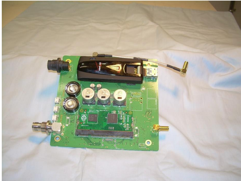
Photograph 17 – View of the PCB with Cell Module Installed
