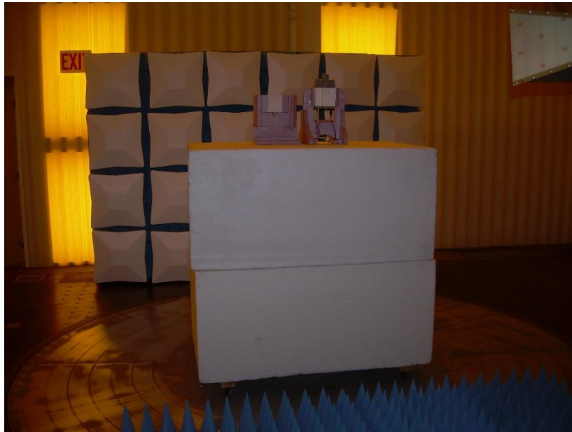
Photograph 6: Radiated Emissions – RE09U Antenna
