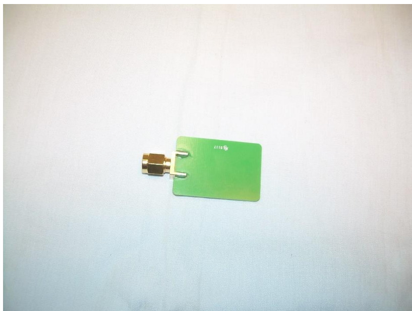
Photograph 27 – View of the Secondary 802.15.4 Transceiver Antenna – Back
