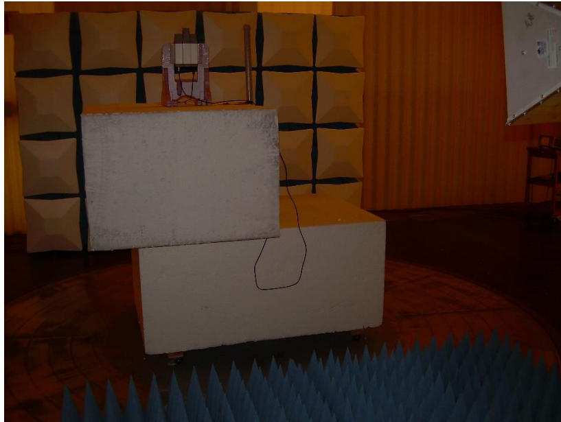
Photograph 7: Radiated Emissions – HG2415U-PRO Antenna
