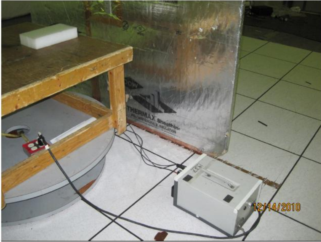
Test-setup photo(s): Conducted emissions
