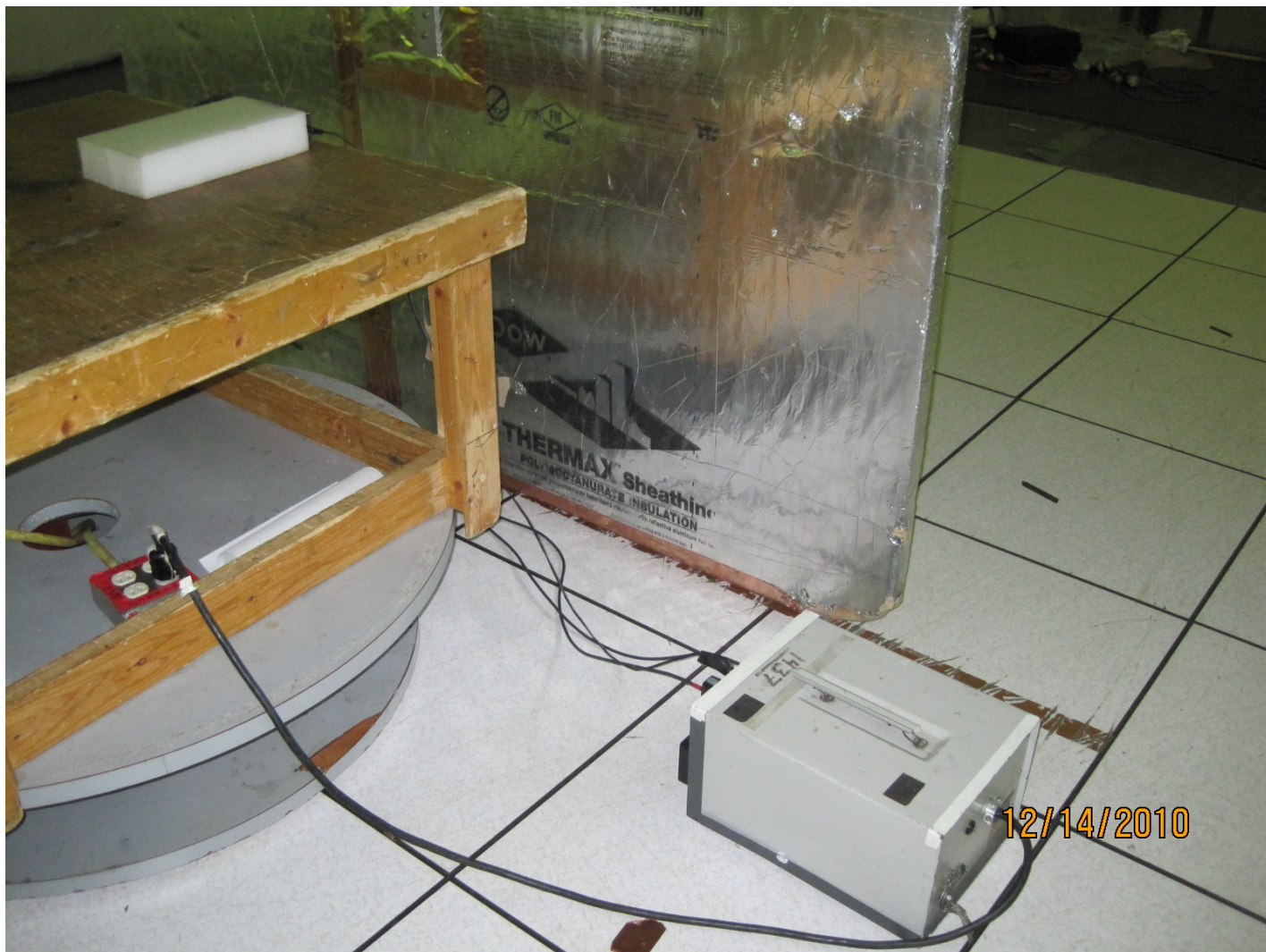
Test-setup photo(s): Conducted emissions
