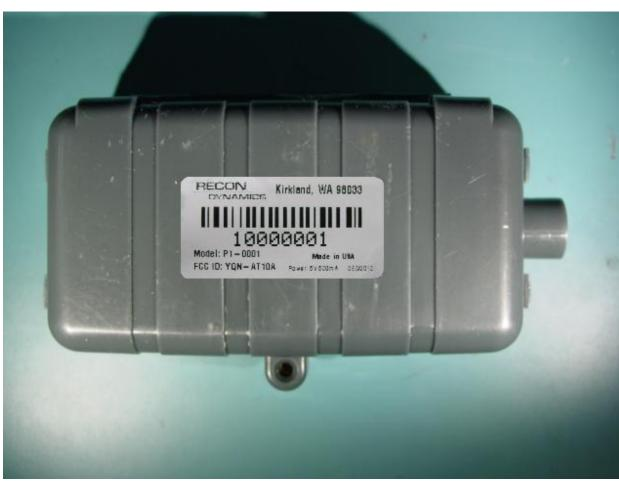
The label will be located on the back side of the product as shown in the picture above. The label is attached to the device with a permanent adhesive.
