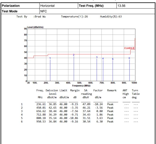
Note 1: Emission Level (dBuV/m) = SA Reading (dBuV) + Factor\* (dB)
