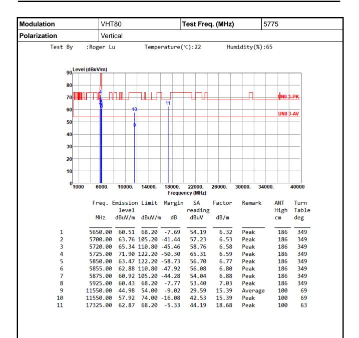
\*Factor includes antenna factor, cable loss and amplifier gain
