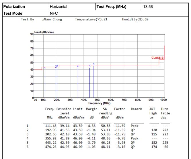
Note 1: Emission Level (dBuV/m) = SA Reading (dBuV) + Factor\* (dB)
