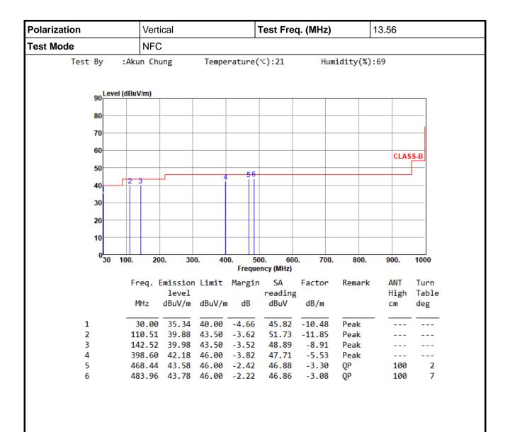
Note 1: Emission Level (dBuV/m) = SA Reading (dBuV) + Factor\* (dB)
