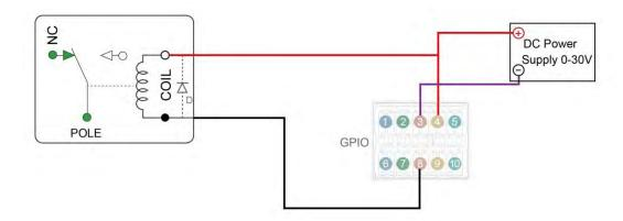
In some cases, you may want WR201 release to automatically press the key to turn on the high-power load, which can be connected according to the following figure:
