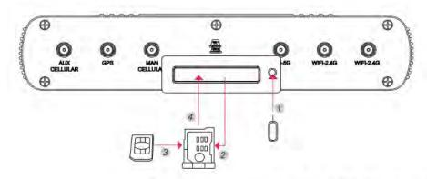
Note: The device is compatible with mini-SIM (2FF) size cards.
