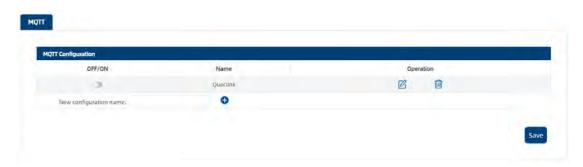
Enter a custom MQTT server name and click the Add icon to create a new MQTT server instance and go to the configuration page. You can click edit button on the right to edit an existing MQTT server instance.
