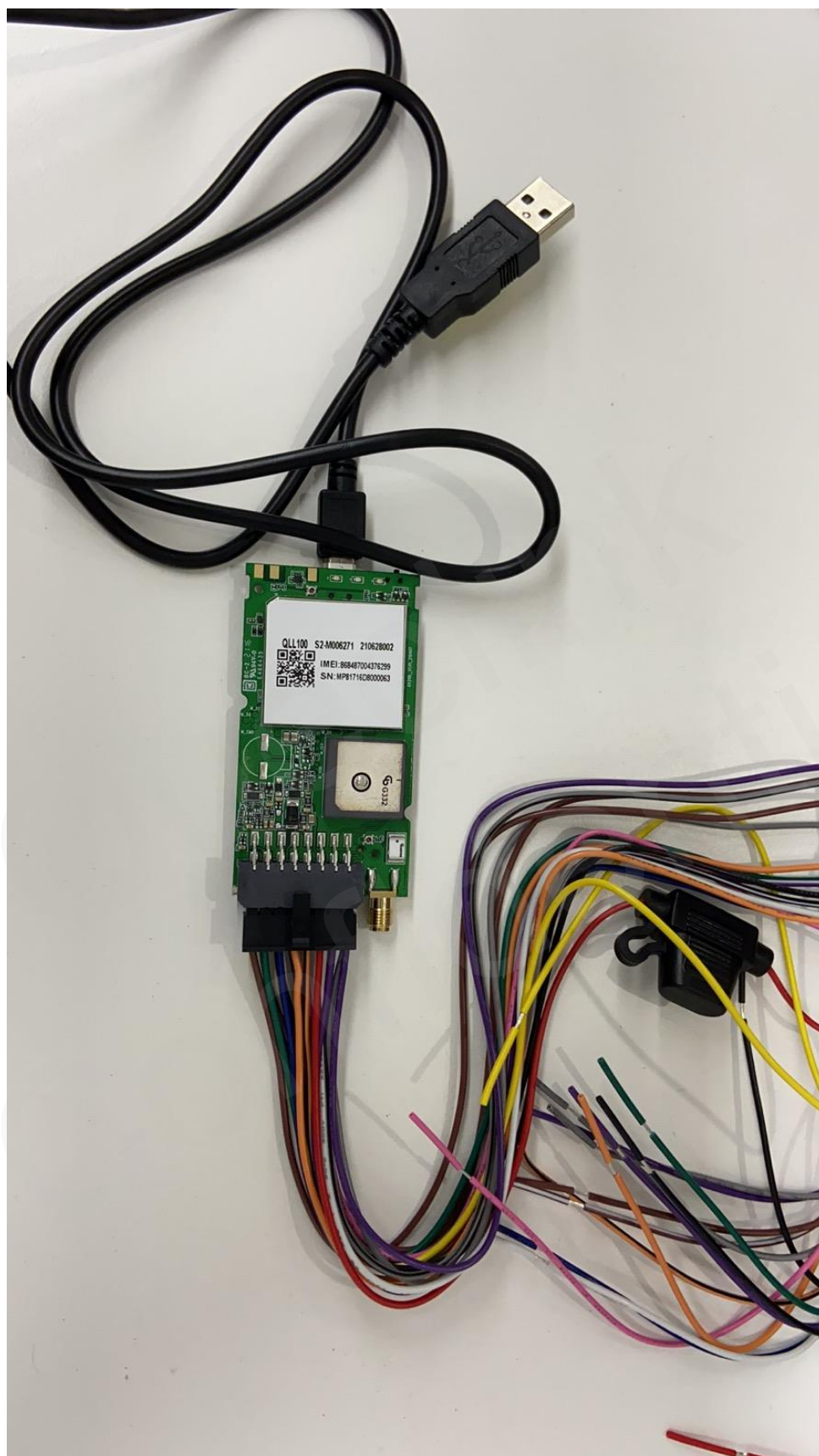
Figure 6. Connect USB with module
