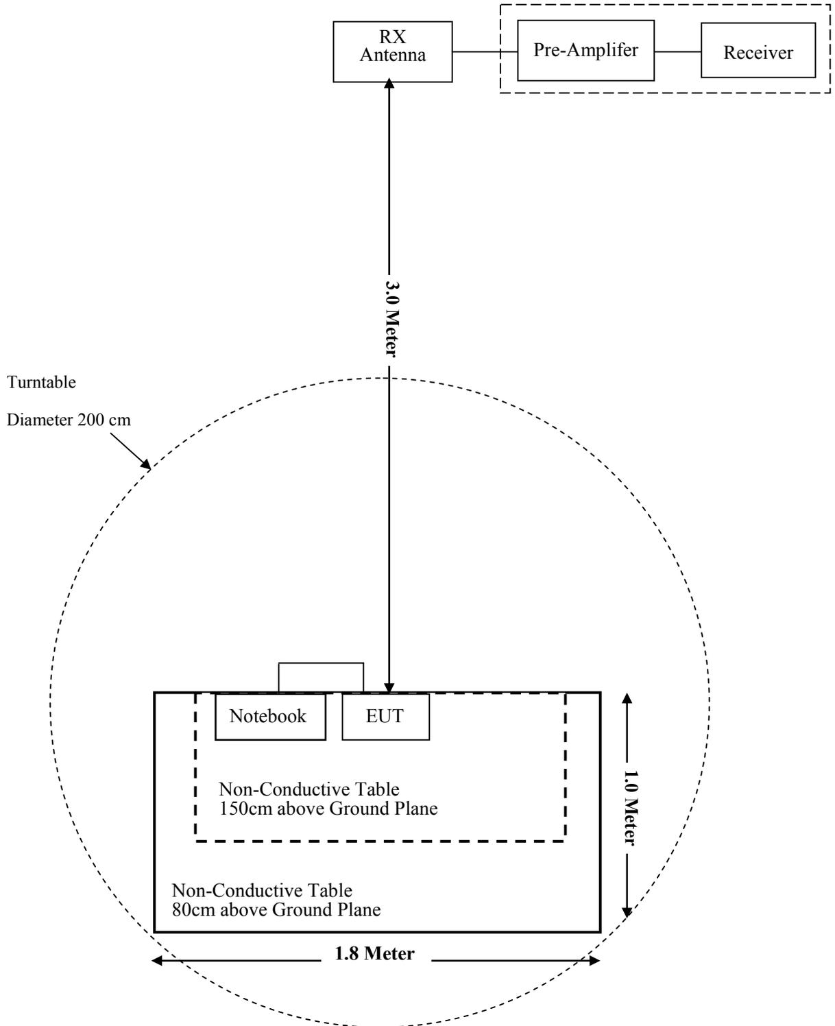
Note: The edge of the test table is in the centre of the turntable in order to keep the EUT in the center of the turntable and to keep the test distance at 3m.
