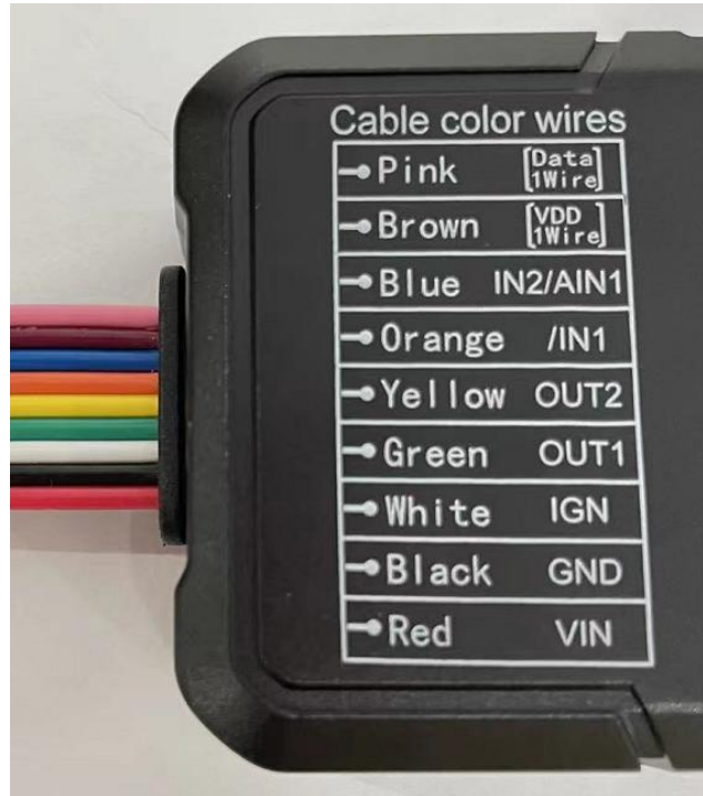
Figure 2: 9-PIN Wire Harness of GV58CEU
