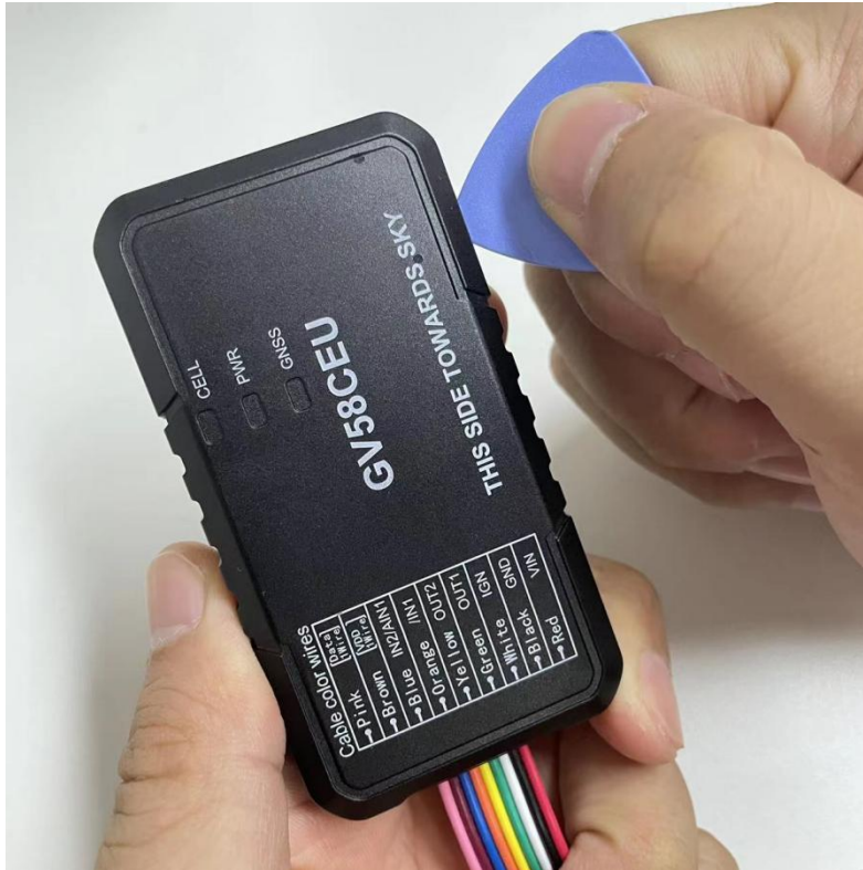
Figure 9: Open the Case
