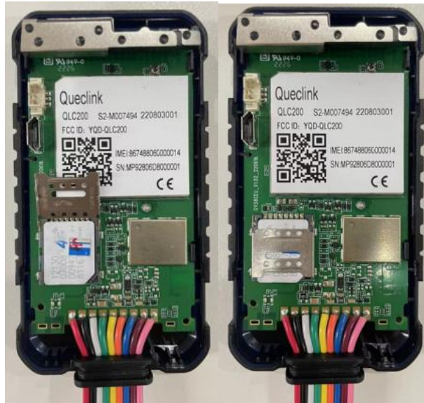
Figure 10: SIM Card Installation
