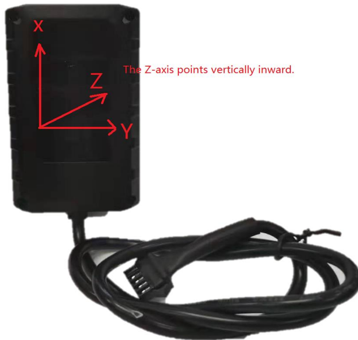
Figure 9. Motion Sensor Direction
