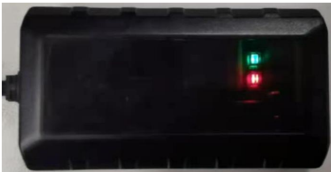
Figure 8. GV57MG V2 LEDs on the Case
