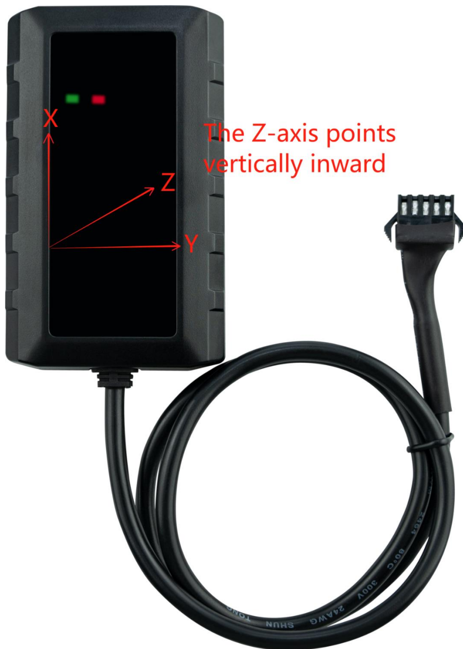
Figure 9. Motion Sensor Direction
