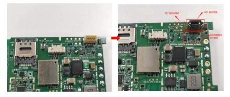
•A 0805 22UF capacitor is added to the DCDC output pin and a feedforward capacitor is
