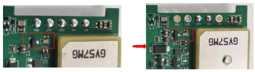
•The original pin is not used. Adding a new ADC pin and adding a bypass capacitor . It will not affect the radio frequency. It is used to detect the charging current and prevent the battery from overcharging.
