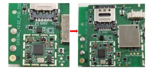
• Replace the GPS receiver from AG3331 with AG3352 and update the peripheral circuit.
