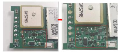
•Change and add two resistors to the MOS tube on the OUT tube
