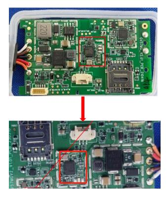
•Bluetooth antenna gain increases to 2.1dbi and the antenna type keep the same.
