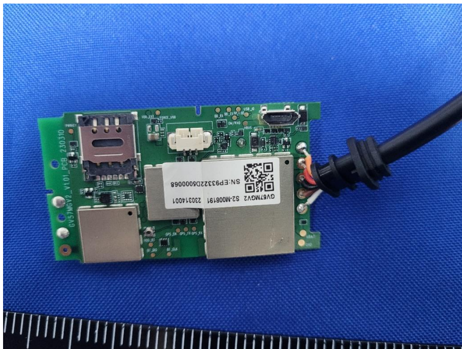
MAIN BOARD REAR VIEW (WITH SHIELDING)
