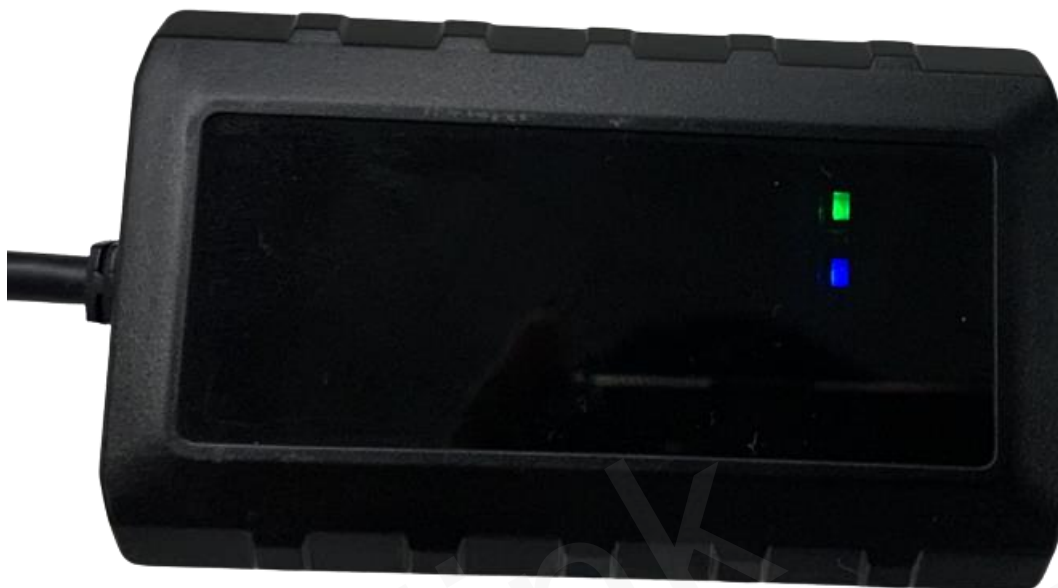
Figure 8. GV57CG LEDs on the Case
