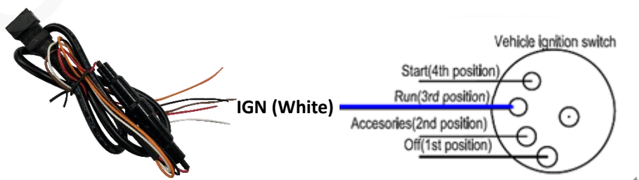
Figure 4. Typical Ignition Detection
