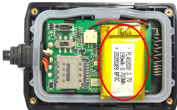
Figure 7. Installing the Internal Backup Battery
