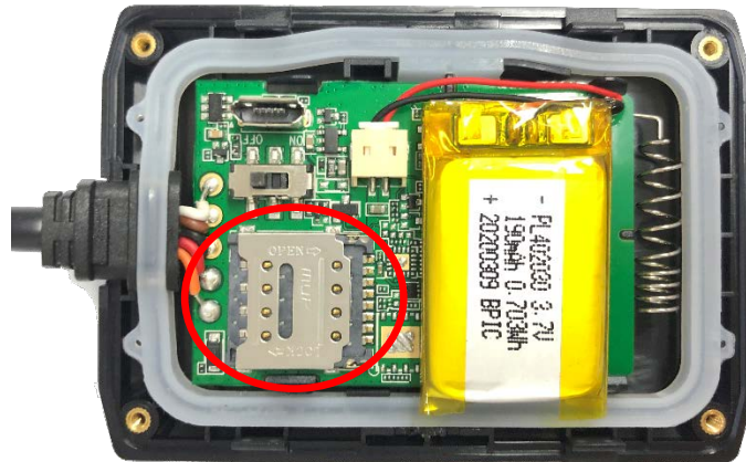
Figure 6. Installing a SIM Card
