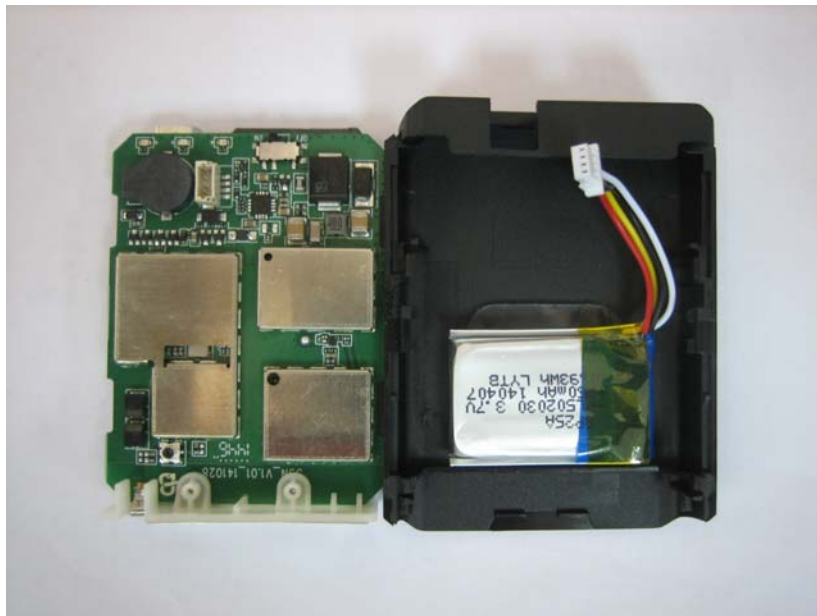
Figure 6. Backup Battery Installation
