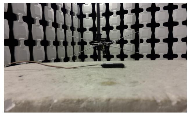
EIRP Test, Radiated Spurious Measurement (Above 1GHz) Setup
