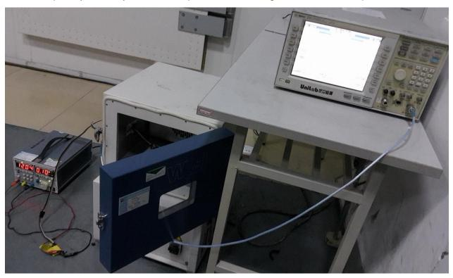
Radiated Spurious Measurement(below 30MHz) Setup
