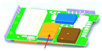
Figure 3. SIM Card Installation
