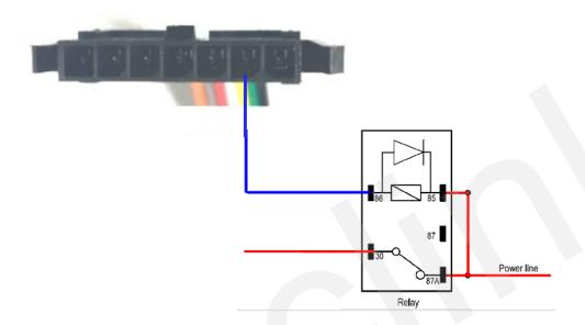
Figure 9: Typical Connection with Relay
