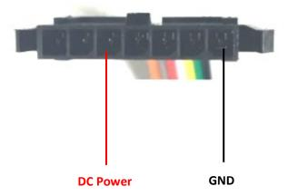
Figure 3: Typical Power Connection
