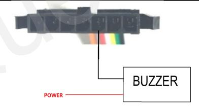
Figure 6: Typical Connection with Buzzer As Digital Output
