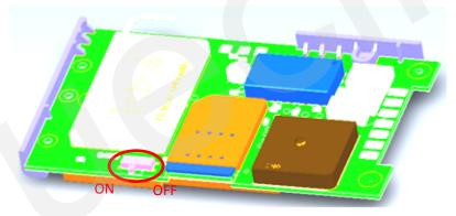
Figure 4. Switch and ON/OFF Position
