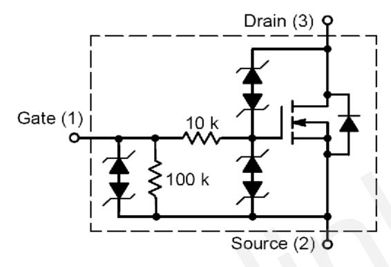
Figure 5: As Digital Output Internal Drive Circuit
