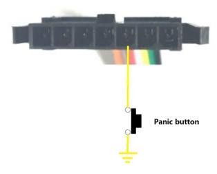
Figure 7: Typical Digital Input Connection
