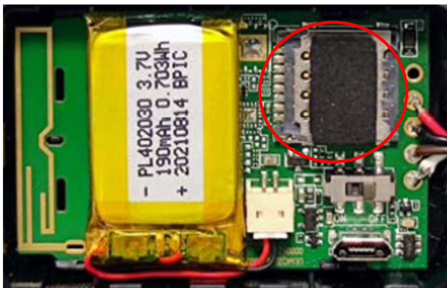
Figure 8. Installing a SIM Card
