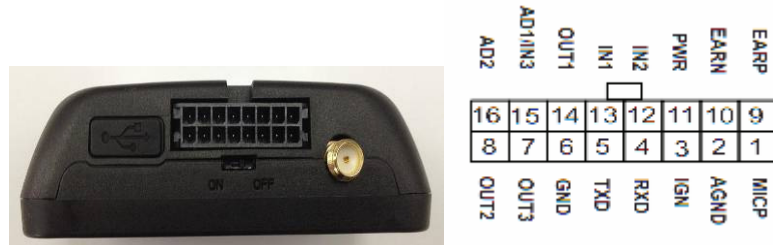
Figure 2. The 16 PIN Connector on the GV304N
