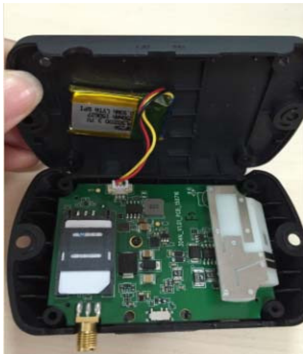
Figure 6. Backup Battery Installation
