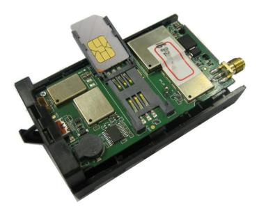
Figure 5. SIM Card Installation
