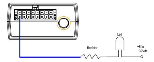
Figure 15. Typical Connection with LED
