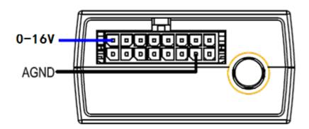
Figure 12. Typical Analog Input Connection
