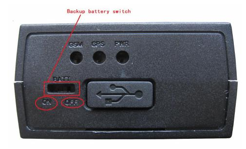
Figure 7. Switch and ON/OFF Position
