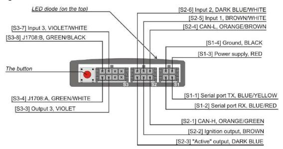
Figure 19. The External Interface of CAN100 Device
