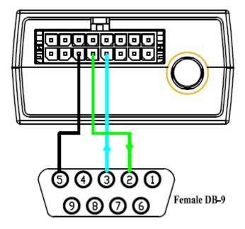
Figure 17. Typical Connection with RS232 Port
