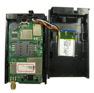
Figure 6. Backup Battery Installation
