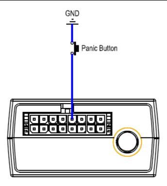
Figure 11. Typical Digital Input Connection
