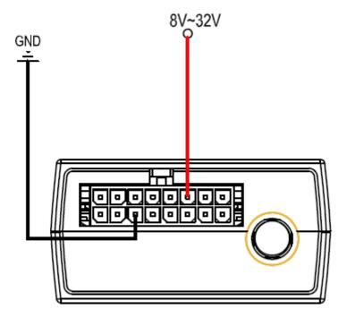
Figure 9. Typical Power Connection
