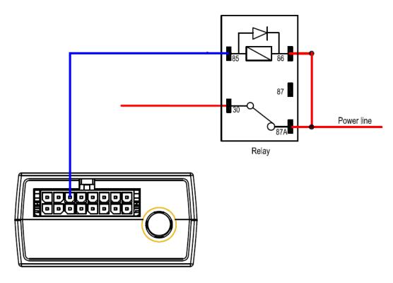
Figure 14. Typical Connection with Relay
