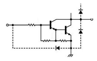
Figure 13. Digital Output Internal Drive Circuit
