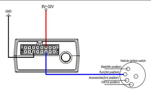
Figure 10. Typical Ignition Detection
