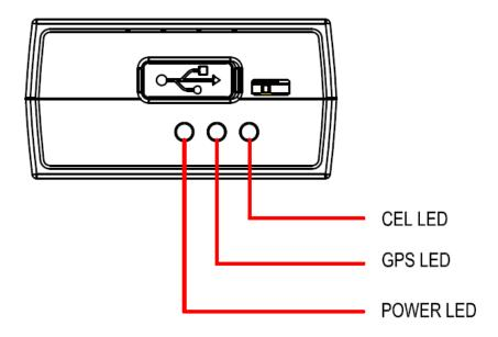
Figure 16. GV300W LED on the Case
