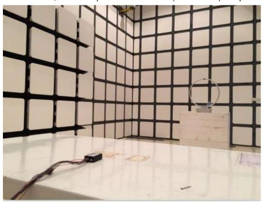
ERP Test, Radiated Spurious Measurement(30MHz to 1GHz) Setup
