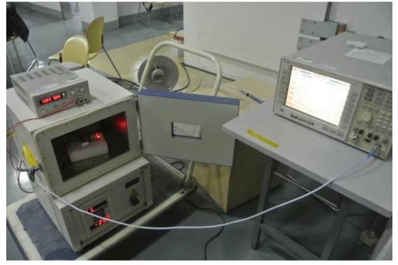
Radiated Spurious Measurement(below 30MHz) Setup
