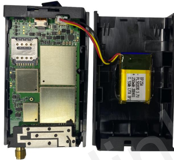
Figure 6. Backup Battery Installation
