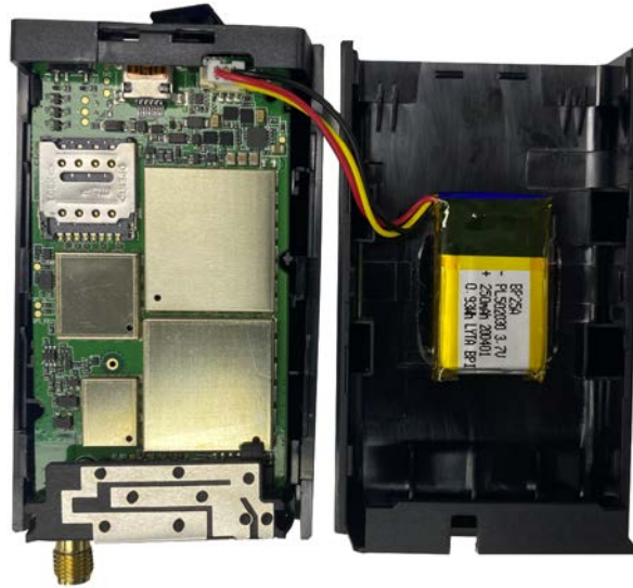
Figure 6. Backup Battery Installation
