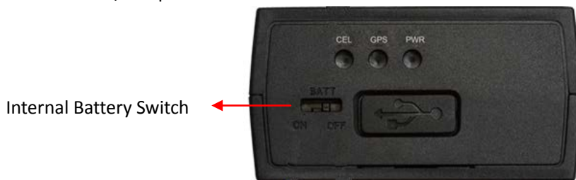
Figure 7. Switch and ON/OFF Position
