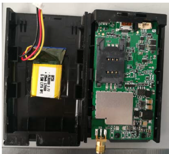
Figure 5. Backup Battery Installation
