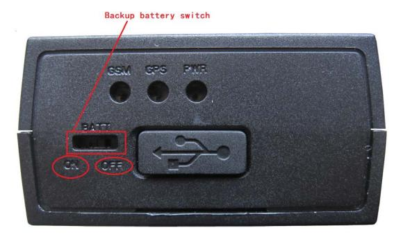
Figure 7. Switch and ON/OFF position
