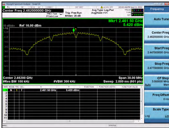
802.11b HIGH CHANNEL, CARRIER LEVEL
