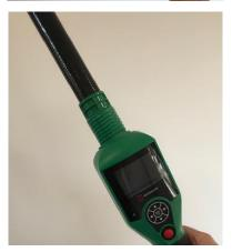
Take a Detachable Antenna and push the connector end of the antenna onto the connector end of the Reader.
