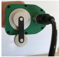
Connect and fasten the Data/Charging Cable to the Data/Charging port on the Reader using a clockwise motion to secure the cable in place.
