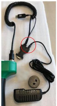
Plug the connector on the cable of the Battery Charger into the socket at the back of the 9 pin serial data connector on the Data/Charging Cable.
