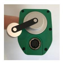
Loosen the data/charging cap on the reader.
