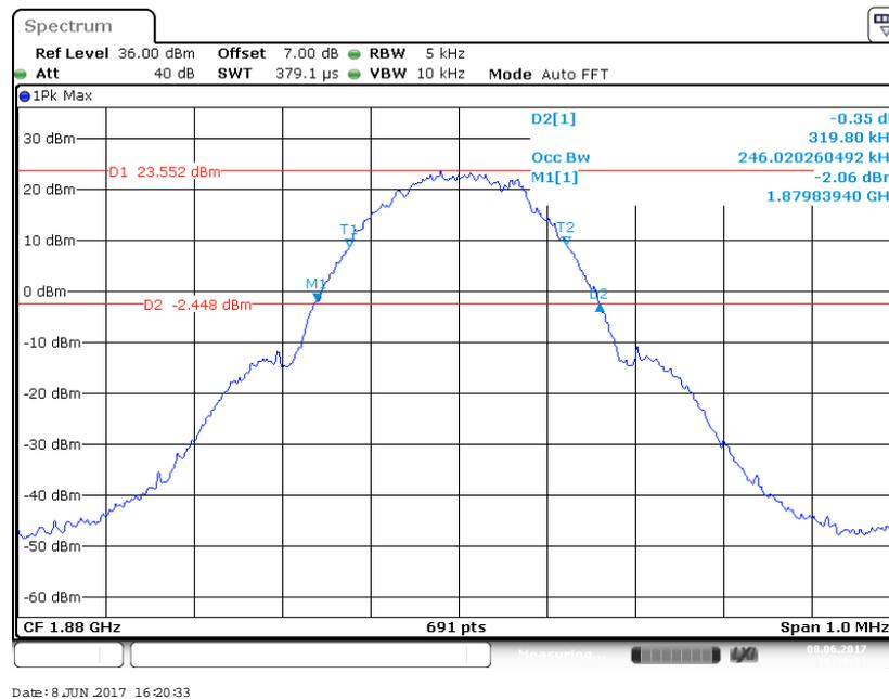
**§ 2.1051; § 22.917 (a);§ 24.238 (a) – SPURIOUS EMISSIONS AT ANTENNA TERMINALS**
