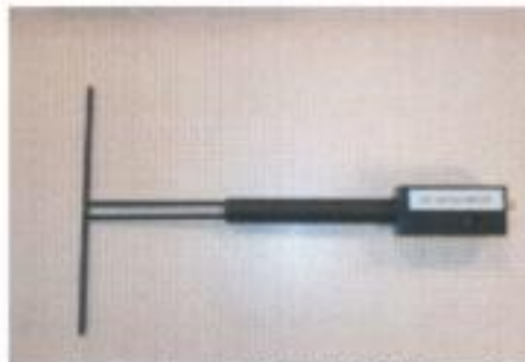
Figure 1 – Satimo COMOSAR Validation Dipole
