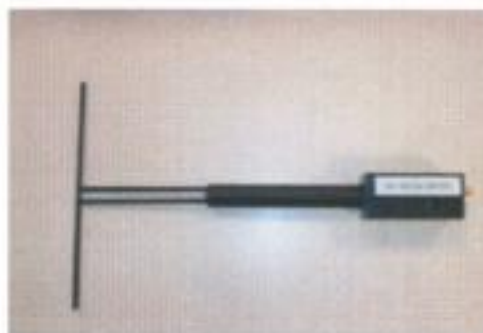
Figure 1 – Satimo COMOSAR Validation Dipole
