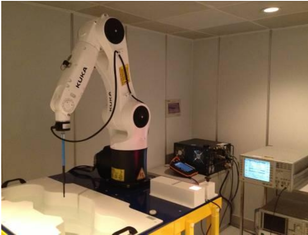
Fig.2COMO SAR Test System
