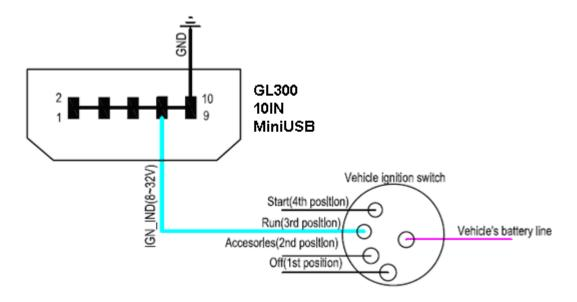
Another easy way is to connect PIN7 to a power output in the fuse box of the vehicle which is only enabled after the vehicle is ignition on. For example: the power output for radio FM.
