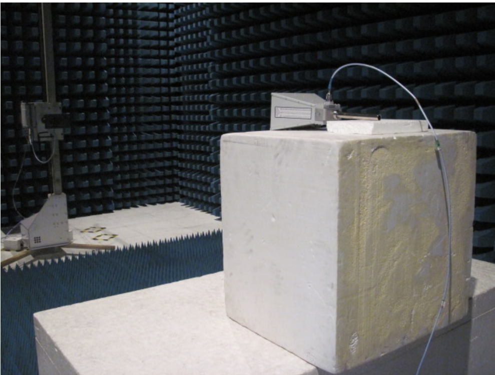
Description: Substitution Antenna for EIRP Test
