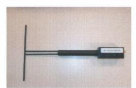
Figure 1 – Satimo COMOSAR Validation Dipole
