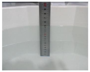
Fig.9 Body Liquid of 1900MHz(15cm)
