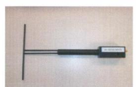
Figure 1 – Satimo COMOSAR Validation Dipole
