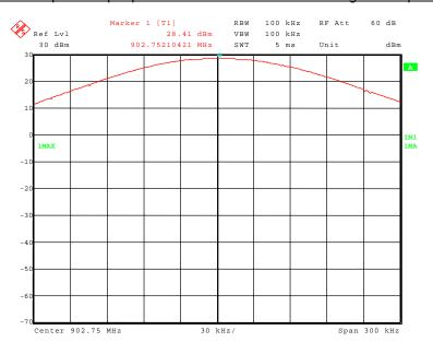
153143 29.wmf: Maximum peak output power at the middle of the assigned frequency band:
