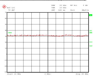
No significant frequencies above the noise floor of the system (max.  $33 \text{ dB}\mu\text{V/m}$  (measured with peak detector) at 3 m distance) were found during the preliminary radiated emission test, so no measurements were carried out on the outdoor test site.
