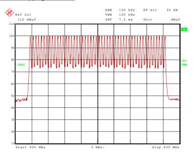
Remark: A smaller Resolution bandwidth was used in order to receive a better optical separation of the signal peaks.
