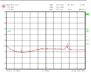
122887\_69.wmf: Spurious emissions from 30 MHz to 200 MHz (operation mode 2):
