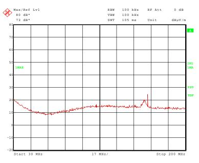
122887\_57.wmf: Spurious emissions from 30 MHz to 200 MHz (operation mode 3):
