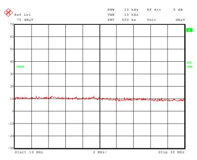
122887\_88.wmf: Spurious emissions from 10 MHz to 30 MHz (operation mode 2):
