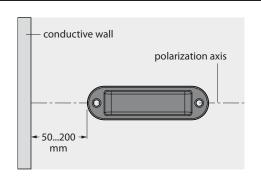
A minimum distance to a conductive wall must be observed for the data carriers. This is 50...200 mm parallel to the polarization axis.
