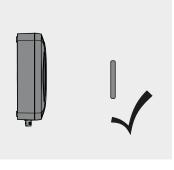
If the data carrier antenna is aligned vertically to the read/write head, this will only result in poor performance and a minimum read range. Vertical alignment should therefore be avoided.
