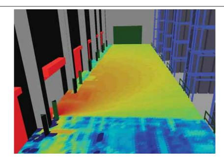
All the essential physical factors involved in the propagation of radio waves are taken into account. These include for example: Attenuation characteristics in air and other media (obstacles), reflection and transmission properties on objects of different materials, polarization characteristics, antenna characteristics and gain of read/write units and data carriers.
