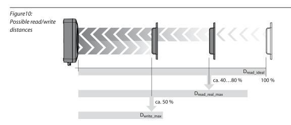
Reserve capacity must be included in planning, not only with regard to the possible radio range, but also with regard to time available for accessing the data carrier on the fly within a time window.
