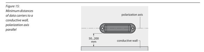
A minimum distance to two conductive walls must be observed for the data carriers. This is 50...200 mm parallel and vertical to the polarization axis.
