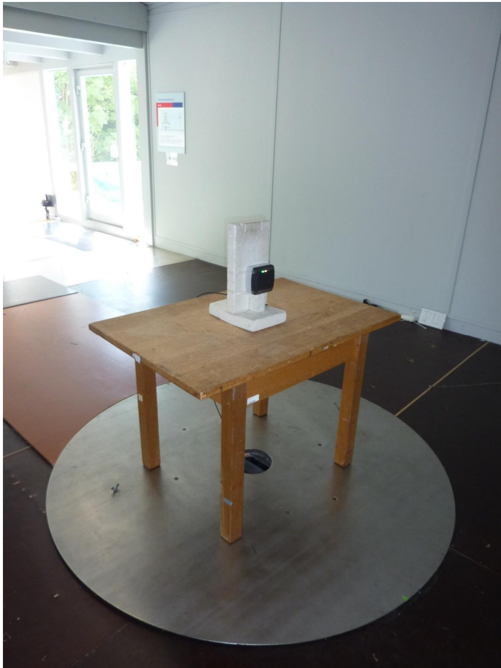
142568_f.JPG: TN902-Q120L130-H1147, test set-up open area test site
