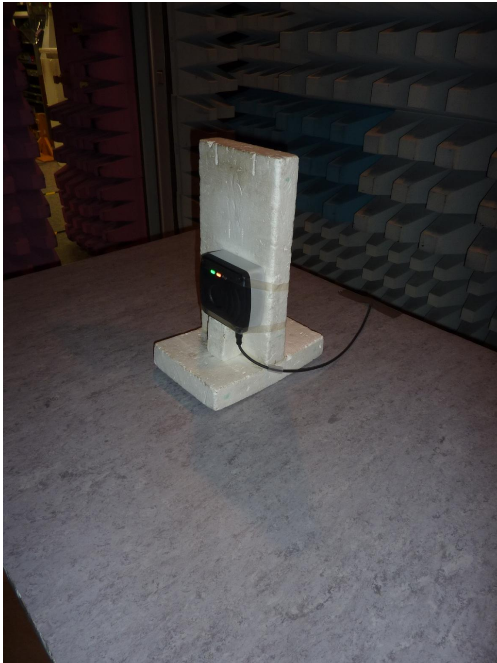
142568_b.JPG: TN902-Q120L130-H1147, test set-up fully anechoic chamber
