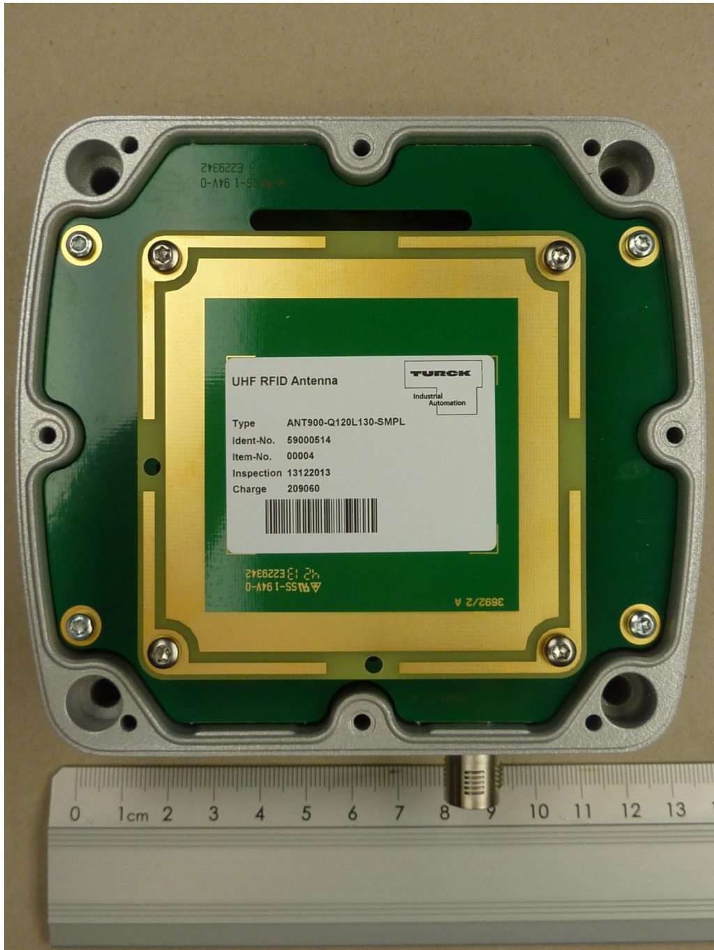
142568_12.JPG: TN902-Q120L130-H1147, internal view 1 (cover removed)
