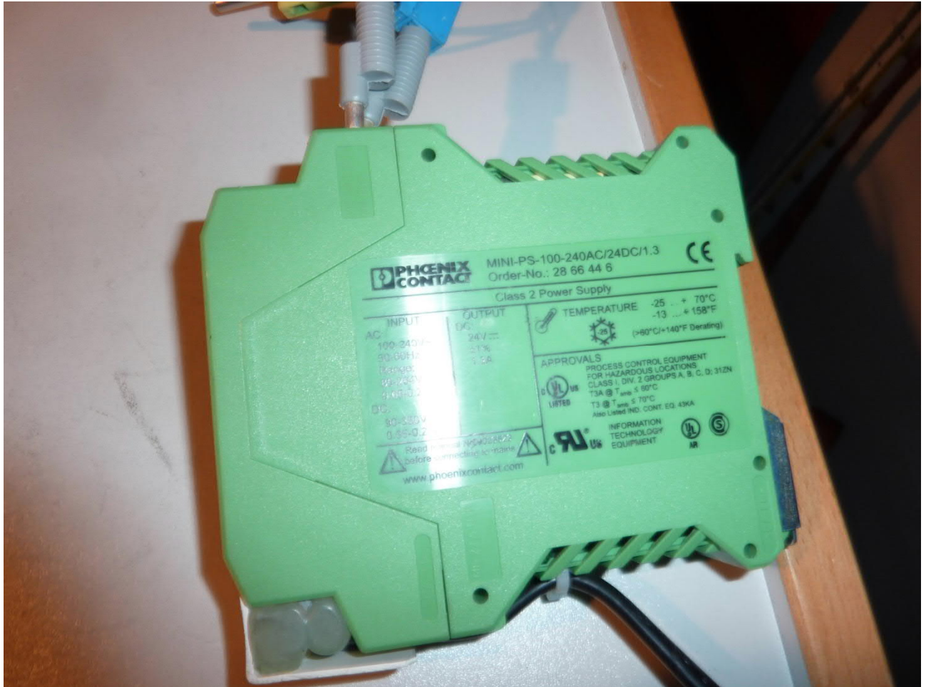
Power adapter MINI-PS-100-240AC/24DC/1.3
