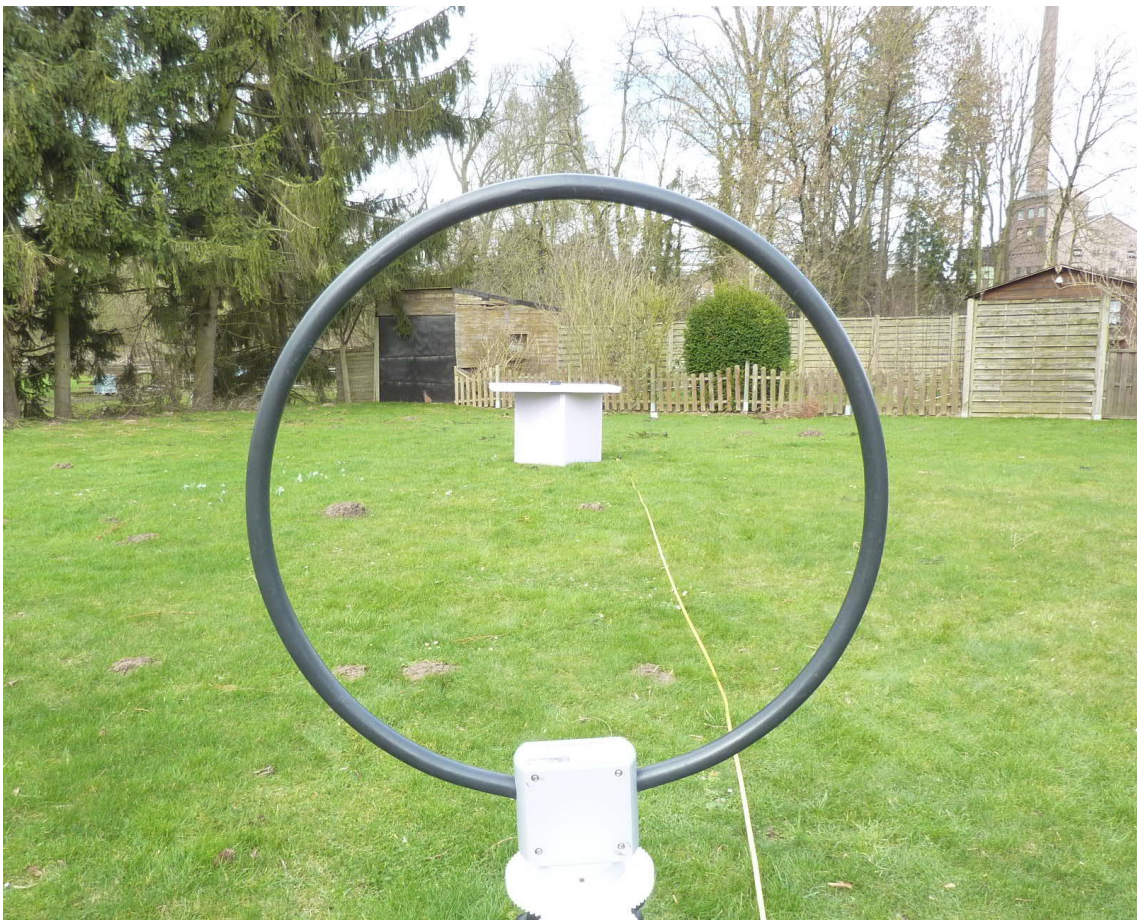
Test setup open area test site (9 kHz to 30 MHz) at 10m distance
