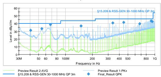
The results of the standard subsequent measurement in a semi anechoic chamber are indicated in the table below. The limits as well as the measured results (levels) refer to the above-mentioned standard while taking account of the specified requirements for a 3 m measuring distance.
