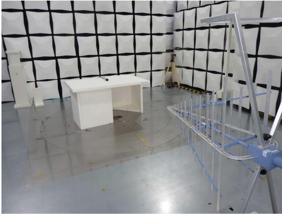
211147_05:Test setup final measurement 30 MHz – 1 GHz
