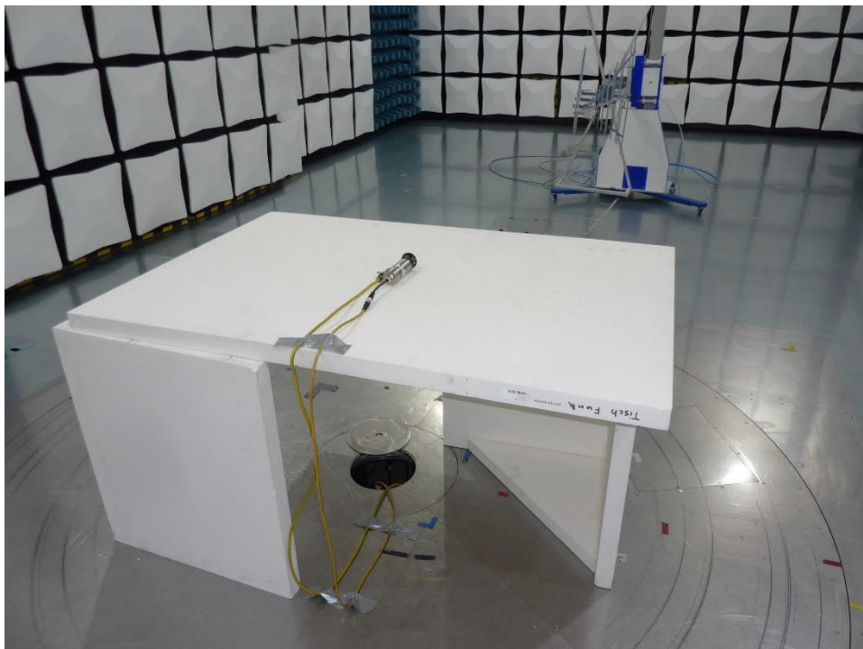
211147_06:Test setup final measurement 30 MHz – 1 GHz
