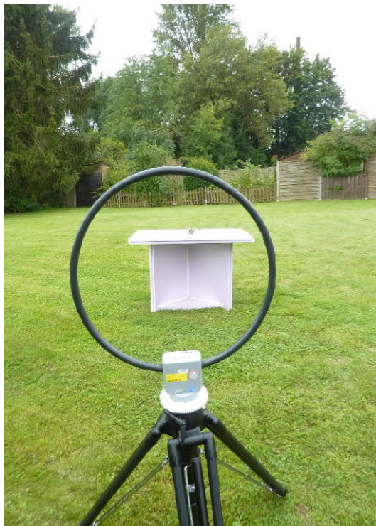
211147_04: Test setup final measurement 9 kHz – 30 MHz
