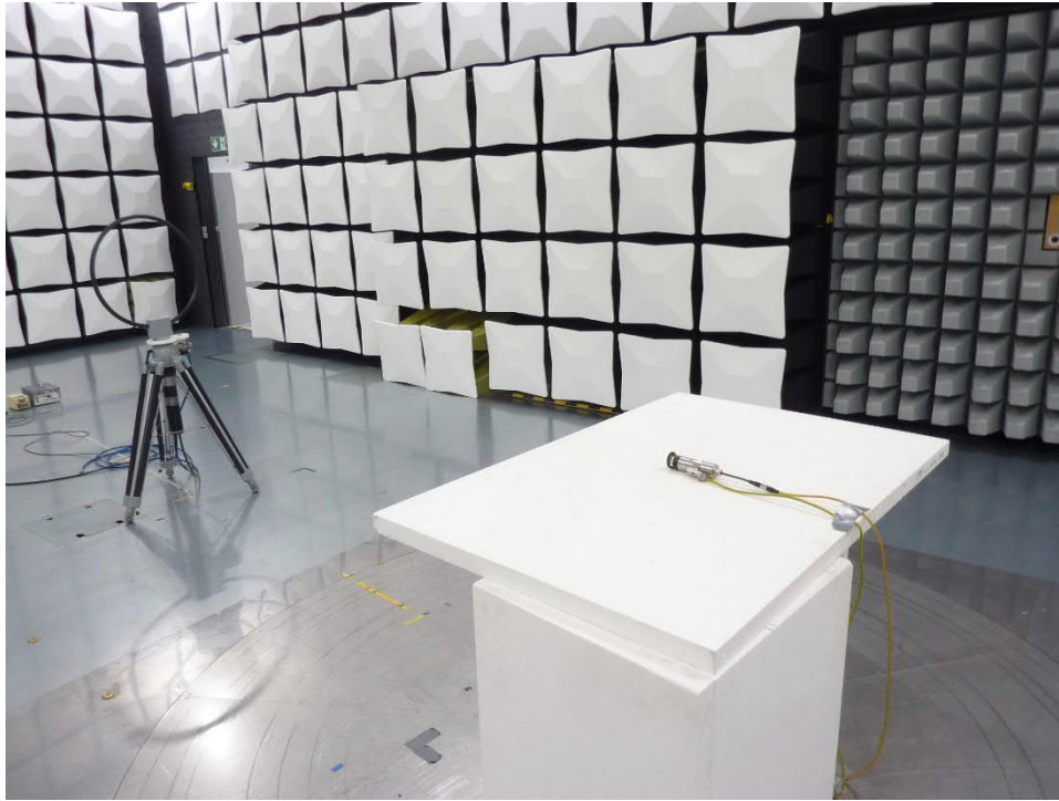
211147_03: Test setup preliminary measurement 9 kHz – 30 MHz
