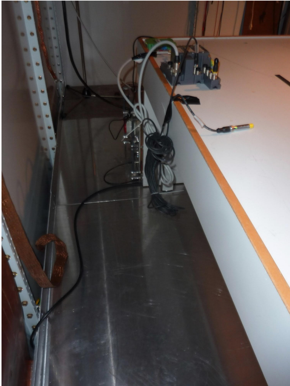
AC Mains conducted emissions test setup
