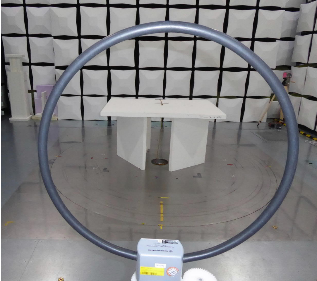
Test setup semi anechoic chamber (9 kHz to 30 MHz)
