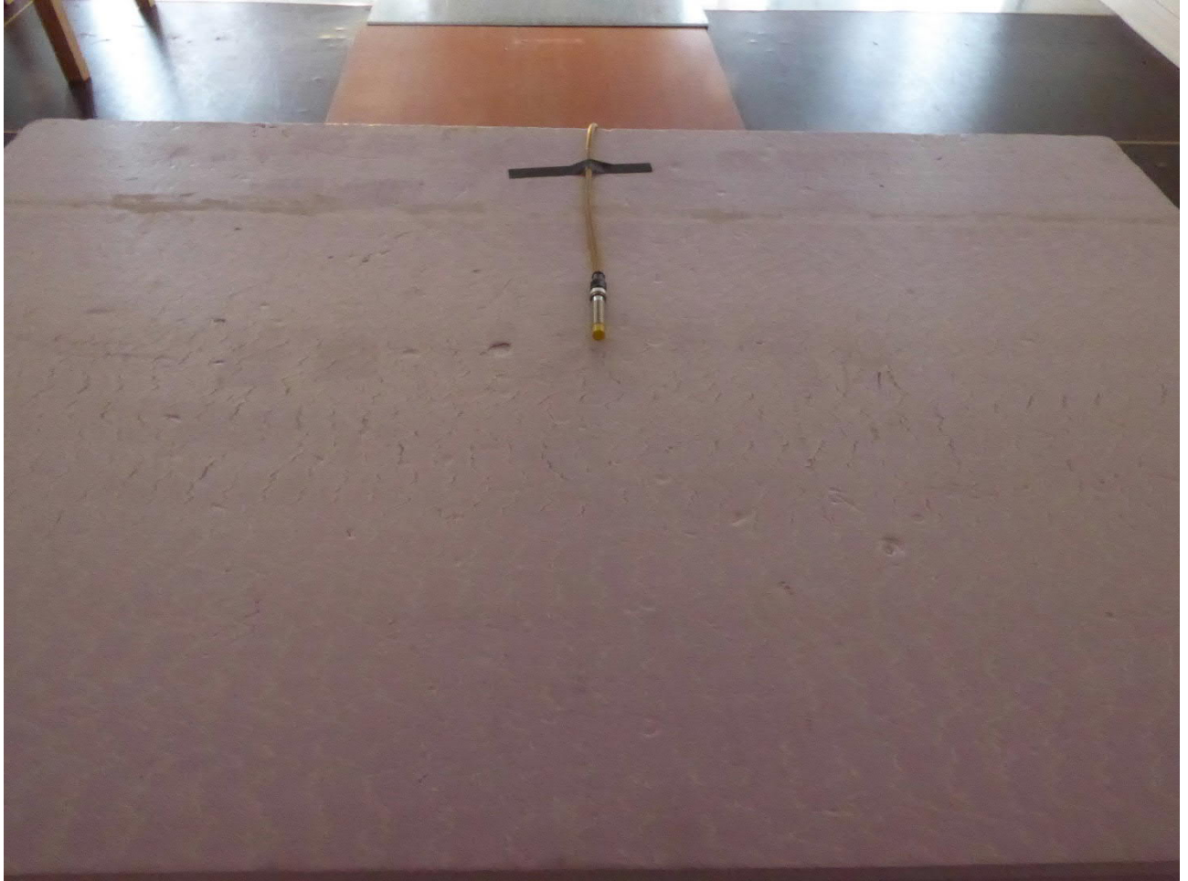
Test setup open area test site (9 kHz to 1 GHz)
