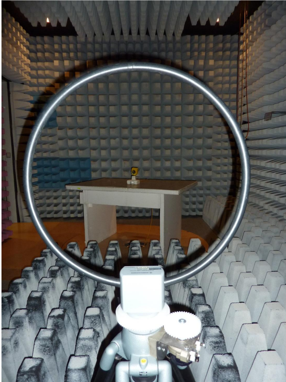
135058_10.JPG: Test setup fully anechoic chamber (H-Field)
