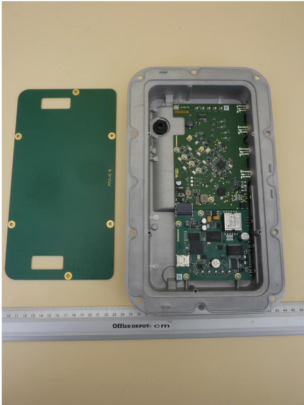
TN-UHF-Q180L300-NA-CDS, internal view 2 (shield removed)
