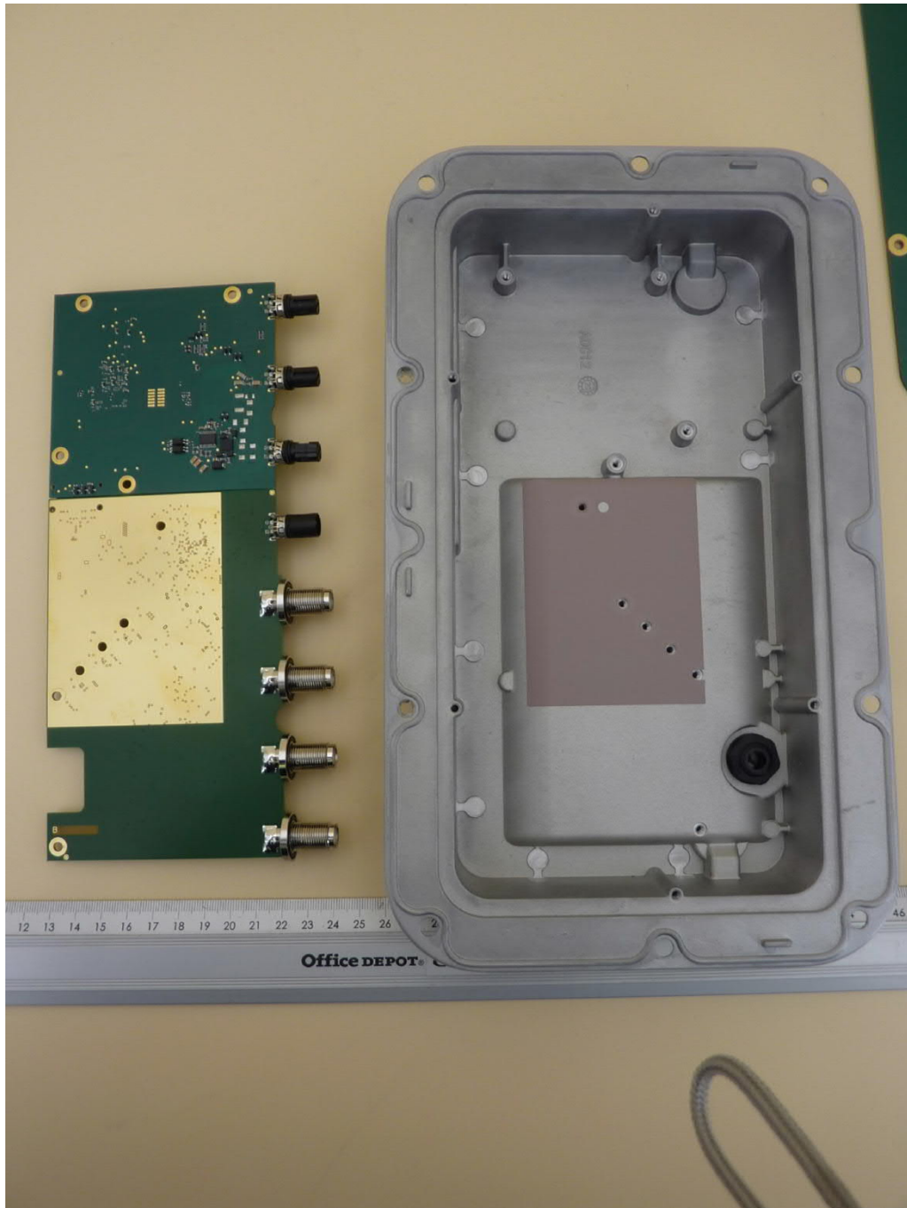
TN-UHF-Q180L300-NA-CDS, internal view 3 (PCBs removed)
